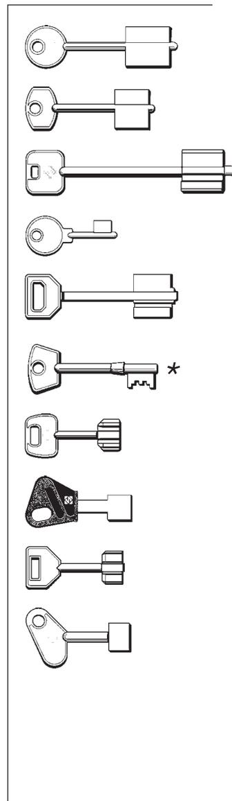
**SINGLE AND DOUBLE BIT, PIN, PIPE AND PUMP KEYS**
