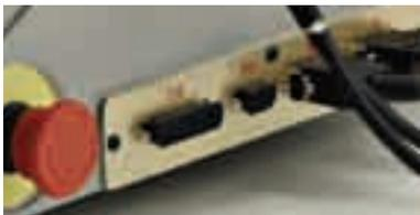
The programs and database on the machine can be updated easily and quickly through a PC serial port.
